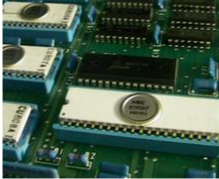
Fig: Several PDIPs and CERDIPs. The large CERDIP in the foreground is an Intel 8080 microprocessor.
